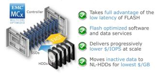
MCx (Multi-Core RAID, Multi-Core Cache and Multi-Core FAST Cache) distributes all VNX data services across all Cores – up to 32. This approach delivers unprecedented application performance while maintaining affordable pricing. Compared to the previous generation, the VNX series with MCx delivers:
