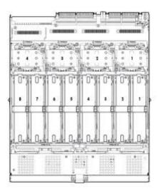
Each memory cartridge contains 12 DIMM slots as shown in figure below:
