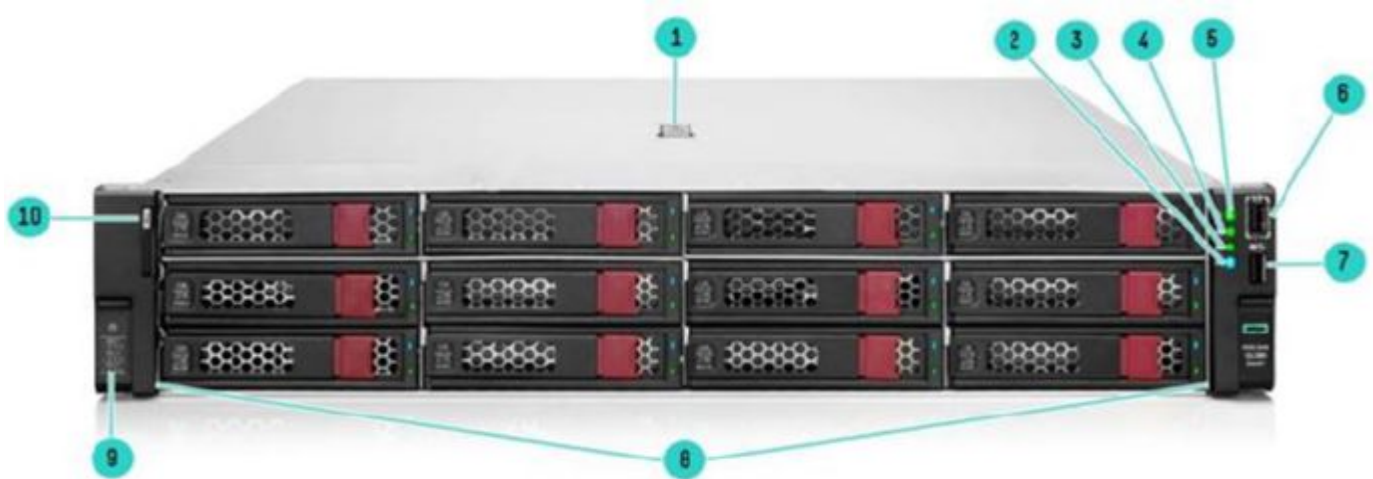
Front View - 12LFF chassis shown
